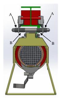
Adjust trolleys so the outside to outside dimension of the trolley is 2" larger than the flange of the beam. Do this by moving the number of washers you have on the inside and outside of the trolley. Be sure that the number of washers are equal on either side of the hoist (inside = inside and outside = outside). Be sure that all washers are put back on to the threaded rod and put back on the side they came from.
